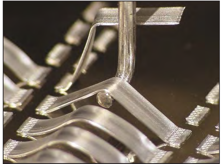
Ribbon pull hook for testing high power ribbon bonds
